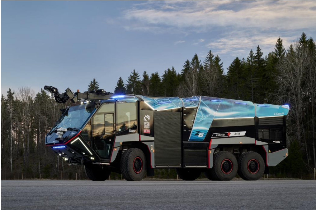
Aircraft Rescue Fire Fighting (ARFF) vehicle with Scania Hybrid powertrain
